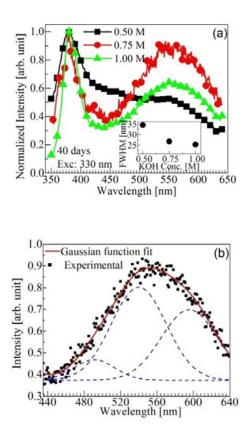
Figure 5: (a) PL spectra of ZnO NPs synthesized for 40 days for different concentrations of KOH. Inset: Variation of FWHM of UV PL peak with the concentration of KOH. (b) Visible PL spectrum fitted with Gaussian functions for the ZnO NPs synthesized for 40 days with 0.75 M KOH.
