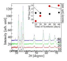
XRD spectra of ZnO NPs prepared using KOH concentration of 1 M for different time (days).
