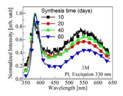
Figure 6: PL spectra of ZnO NPs synthesized using 1.0 M of KOH for different days of synthesis duration.
