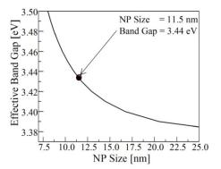
Figure 4: Variation of the effective bandgap of ZnO NPs as a function of NP size according to EMA model. The filled circle is the measured average size of ZnO NP corresponding to bandgap of 3.44 eV.
