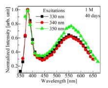
Figure 8: PL spectra of ZnO NPs synthesized for 40 days using 1 M of KOH for different excitations.
