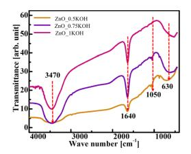
Figure 3. shows the FTIR spectra of ZnO NPs for different KOH concentrations viz 0.5 M, 0.75 M, and 1.0 M.
