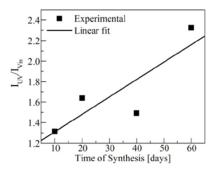
Figure 7: Variation of the intensity ratio of UV to visible emissions of ZnO NPs with the time of synthesis. The solid line is the linear fit to the experimental data points.
